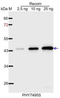
Recom: 2.5 ng, 10 ng and 25 ng recombinant protein containing the peptide for immunization and having a molecular mass of 43 kDa. Electrophoresis: 12% SDS-PAGE Transfer: blotting to NC (nitrocellulose) membrane for 1 h.
