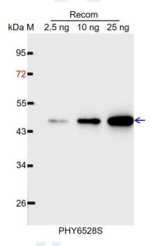
Recom: 2.5 ng, 10 ng and 25 ng recombinant protein containing the peptide for immunization and having a molecular mass of 47 kDa. **Electrophoresis:** 12% SDS-PAGE **Transfer:** blotting to NC (nitrocellulose) membrane for 1 h. **Blocking:** 5% skim milk at RT or 4°C for 1 h. **Primary antibody:** 1:1000 dilution overnight at 4°C.
