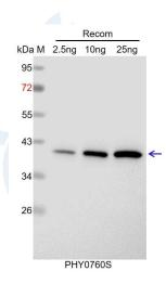
Recom: 2.5 ng, 10 ng and 25 ng recombinant protein containing the peptide for immunization and having a molecular mass of 40 kDa. Electrophoresis: 12% SDS-PAGE **Transfer:** blotting to NC (nitrocellulose) membrane for 1 h. **Blocking:** 5% skim milk at RT or 4°C for 1 h. **Primary antibody:** 1:1000 dilution overnight at 4°C. Secondary antibody: 1:10000 dilution using Goat Anti-Rabbit IgG H&L (HRP) (Cat# PHY6000). Detection: using chemiluminescence substrate and image were captured with
